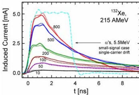
Figure 1: Original TCS obtained in the bias range  $10\text{V} \leq |V_D| \leq 800\text{V}$  from  $^{132}\text{Xe}$  ions of 215 AMeV (solid and dotted lines). A  $^{241}\text{Am}$ - $\alpha$ -transient (dashed line) represents the ‘small-signal case’ at ‘single-carrier drift’. (see text)
