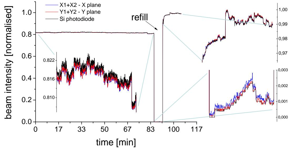
Beam intensity monitoring @ Proxima 1 Soleil (X1+X2) scCVD-PSD 300  $\mu\text{m}$
