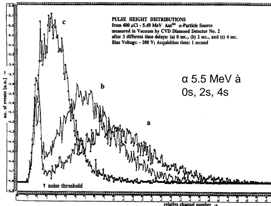
Fig. 3. Pulse height distributions. From 400  $\mu\text{Ci}$ -5.49 MeV  $\text{Am}^{241}$   $\alpha$ -particle source measured in vacuum by CVD diamond detector No. 2 after 3 different time delays: (a) 0 s (b) 2 s and (c) 4 s Bias voltage: -200 V; acquisition time: 1 s. Note, vertical scale is not the same for every PHDs, but individually adjusted to allow a better estimate of PHD peak positions.
