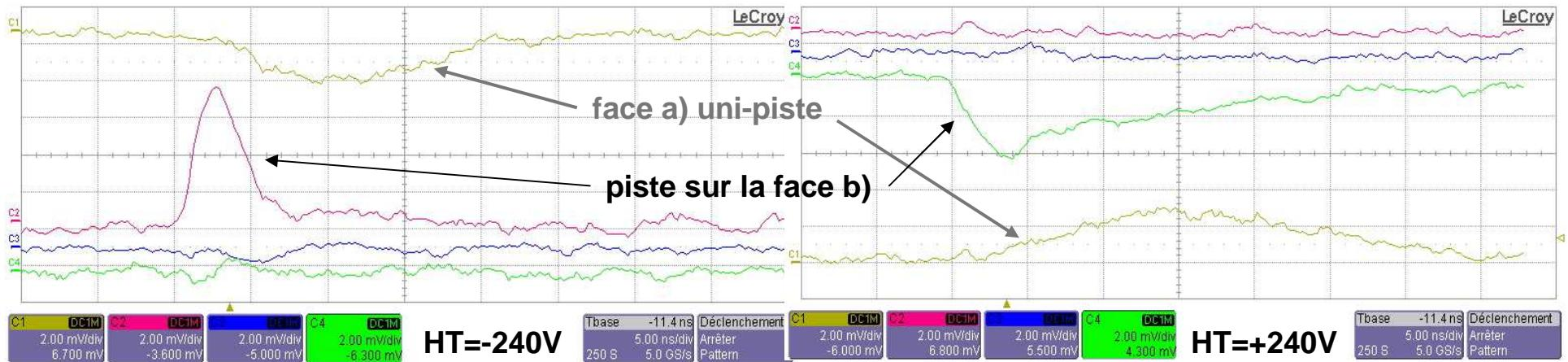
Signals induced by  $^{36}\text{S}$  of 7.2 AMeV in the detector III of ELS type
