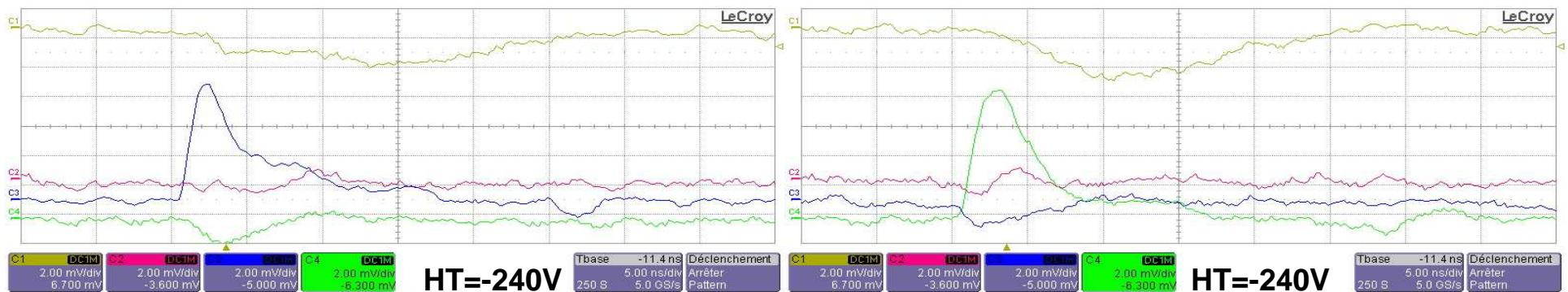
Signals induced by  $^{36}\text{S}$  of 7.2 AMeV in the detector III of ELS type: examples of cross-talk between neighbouring strips on the irradiated face (blue and green)
