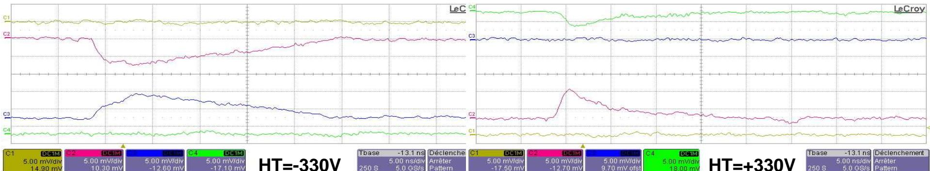
Signals induced by  $^{36}\text{S}$  of 7.2 AMeV in the detector IV of ELP type
