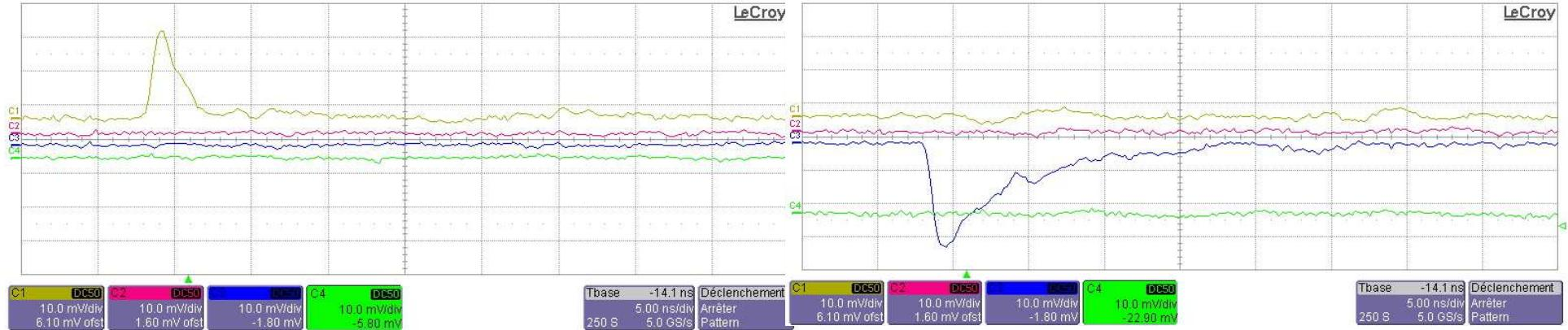
Signals from the strip no. 9 of the face a) - left (yellow curve) and from the strip 9 of the face b) - right (blue curve), amplified with the new preamplifier PRL developed at LPC; the signals were induced by the  $^{70}\text{Zn}$  ions of 8.7 AMeV in the detector IV of ELP type for a voltage of -300 V applied on the face a) (growth), irradiated
