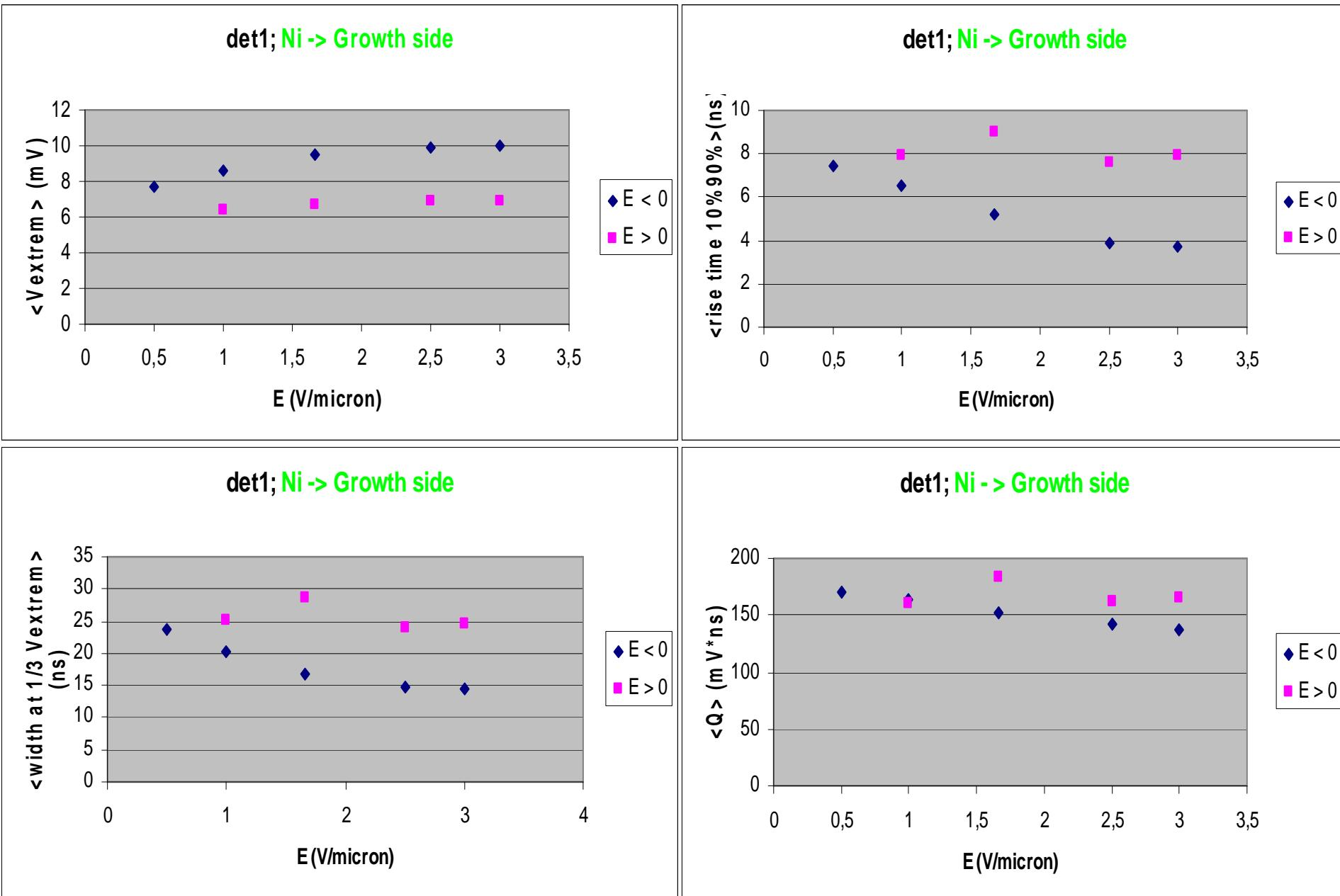
When  $R < d$ , the signal is higher and faster when the **electrons** drift on a **longer way** than the **holes**.
