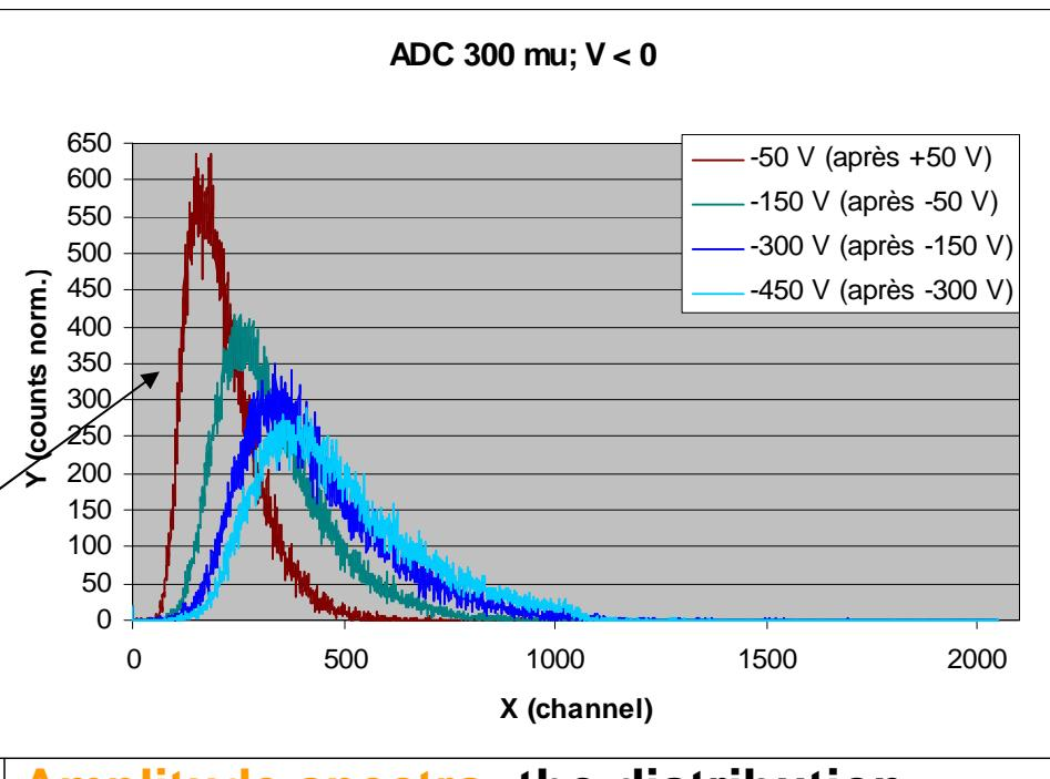
**Amplitude spectra: the distribution becomes narrower when the electric field diminishes.**
