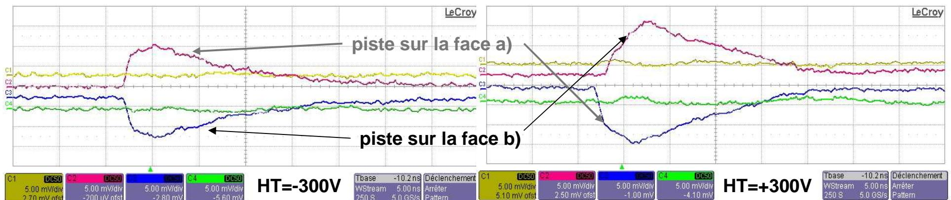
Signals induced by  $^{70}\text{Zn}$  of 8.7 AMeV in the detector IV of ELP type
