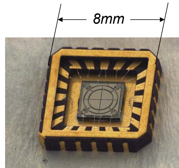
E6 SC diamond in ceramic mount before PCB assembly.  $389\mu\text{m}$  thick,  $50\mu\text{m}$  isolation cross, 3mm hole under the diamond for beam passage.
