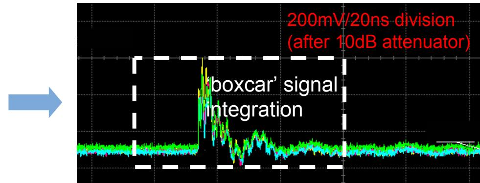
*signal direct to DSO: poor decoupling and 50Ω matching → signal 'bounce'*
