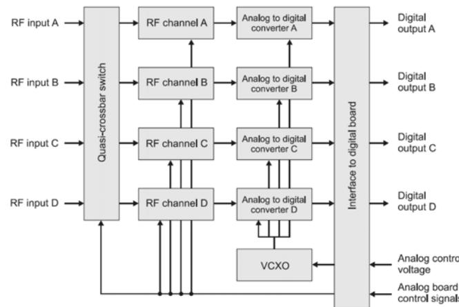
*analog stage: tuned filter (352 or 500MHz)*
