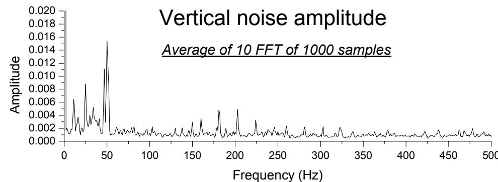
FFTs using Femto DLPCA-200 current preamps
