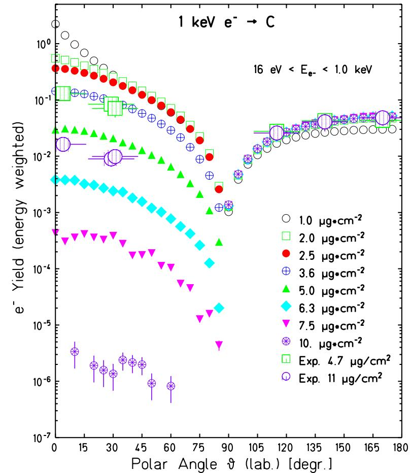
Measured and simulated spectra of electrons from a carbon target bombarded with 1 keV electrons
