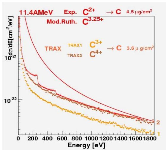
Electrons emitted in collisions of  $\mathbf{C}^{2+}$  projectiles with C, Ni, Ag, and Au targets.
