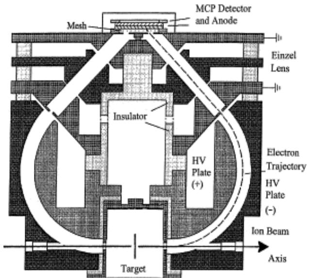
The spectrometer is rotationally symmetric. Electrons emitted in the plane perpendicular to the symmetry axis are energy and angle analyzed.
