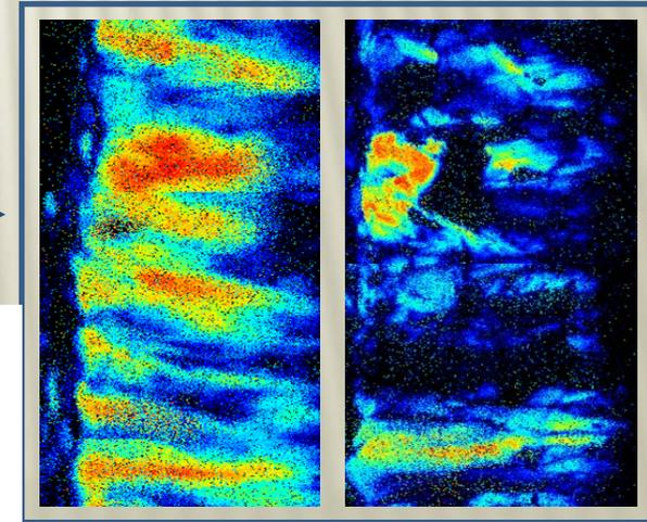
**IBIC** - single ion technique for imaging of microscopic distribution of charge transport properties !
