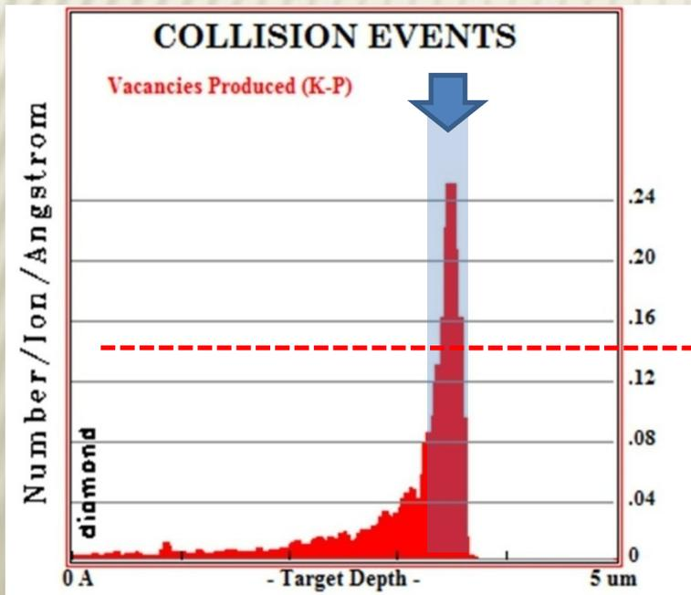
$< 9 \cdot 10^{22} \text{ cm}^{-3} \rightarrow$  (partial) recovery of pristine structure upon thermal annealing
