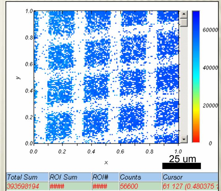
Transmission image of 11 MeV  $C^{3+}$  through Cu grid
