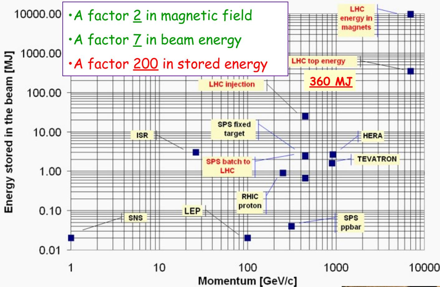
Large damage potential from uncontrolled beams means that comprehensive protection system is needed
