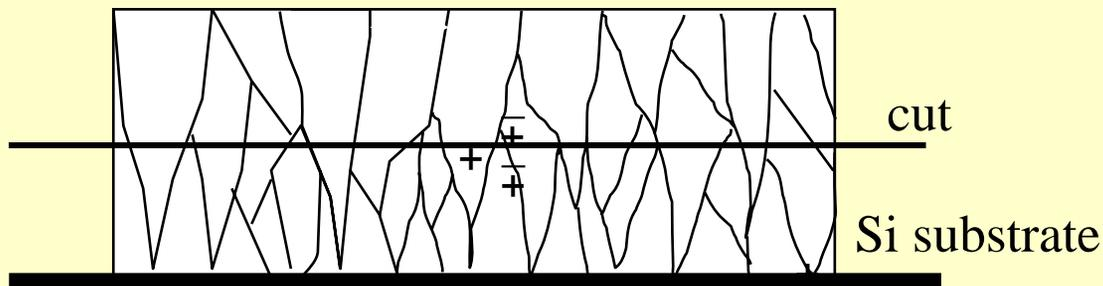
1. two step growth, polishing, round shaped corners, (less stress, larger grains)
